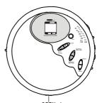
2.) Slide the CD door **OPEN** switch to the right to unlock
